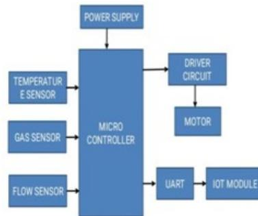
Fig. 3. Block diagram of steam trapping and wireless monitoring of steam.
