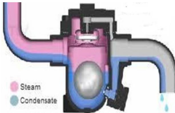
Fig. 2. Working of a steam trap
