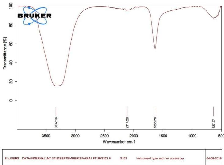
**Figure 4: FTIR Spectrum of Silver Nanoparticles Synthesised by Methanol Extract of *Cassia fistula* and *Manilkara zapota***
