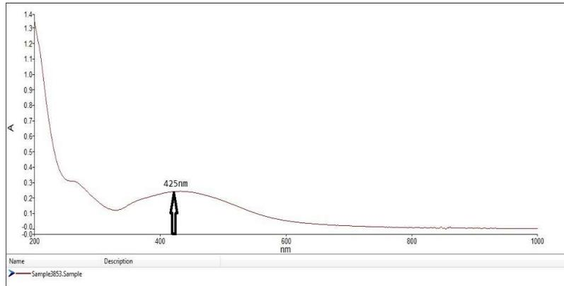
**Figure2: UV-vis Spectroscopy of Silver Nanoparticles by Methanol Extract of *Cassia fistula* and *Manilkara zapota*. Absorption Peak was Noted to be at 425nm.**
