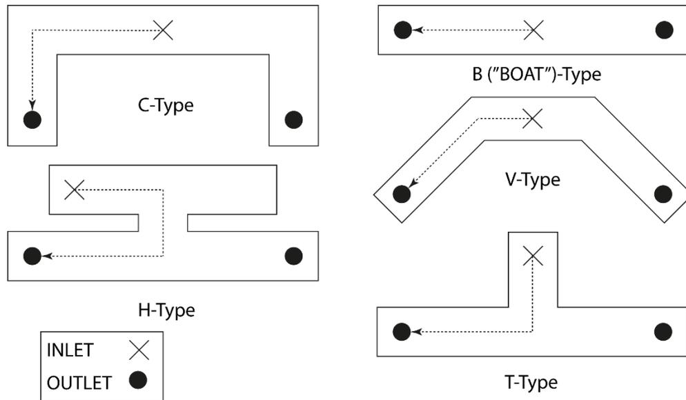
**Fig. 1.** Plan views of different tundish shapes with inlet and outlet locations [5].
