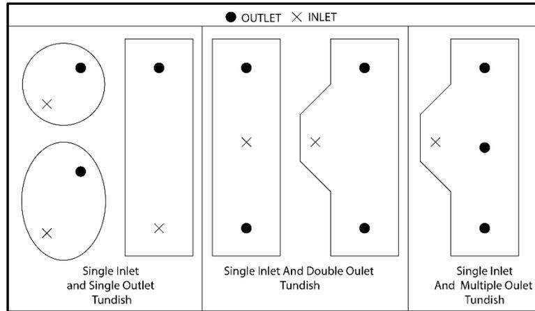
**Fig. 1** Types of tundish based on number of inlets and outlets [41]
