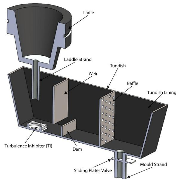
**Fig. 3** Schematic representation of tundish with some flow modifiers [5]
