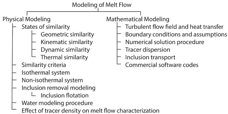
**Fig. 2** Melt flow modeling approaches classification for tundish [5]
